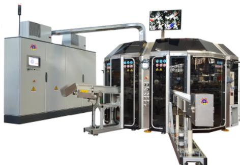
The MHM is a fully servo assisted silkscreen printer suitable for continuous decoration on round, elliptical and flat objects.
