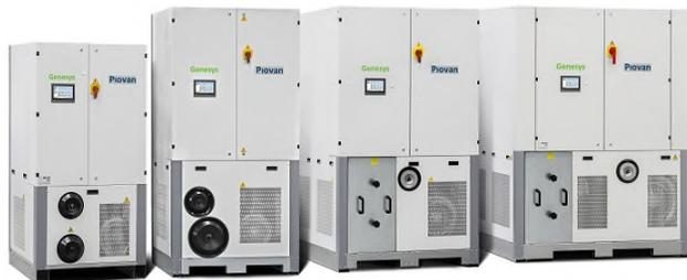
The new Genesys line of auto-adaptive single hopper drying systems from Piovan delivers optimal and consistent operating conditions and lower energy consumption. It is one of the first patent issued in Europe for a high-efficiency polymer drying system.
