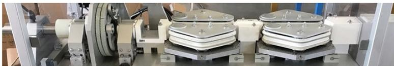
The range of machines built by BARUFFALDI Plastic Technology-Primac has been enriched with the new TC.TVP/40 planetary cutter with built-in traction haul-off, for cutting and evacuating medical pipes directly from
